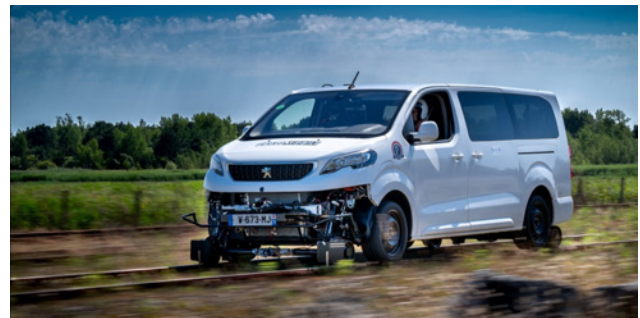
The Ferromobile road-rail vehicle validated for open-track trials
